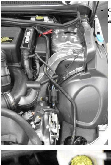
Connect ground to bolt as shown (enlarge opening if needed on around connector)
